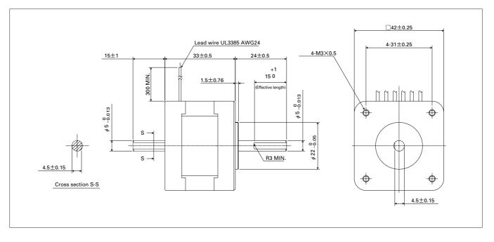
Fig. 2 External dimensions of the 2-phase 42mm Sq. 0.9° stepping motor "SANMOTION F"
