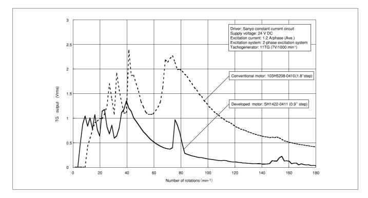
Fig. 4 Comparison of Speed Fluctuations in Basic Step Angle  $0.9^{\circ}$  and  $1.8^{\circ}$
