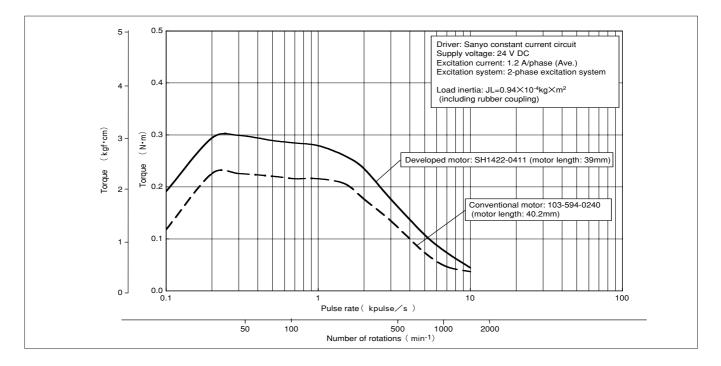
Fig. 5 Comparison of Torque Characteristics
