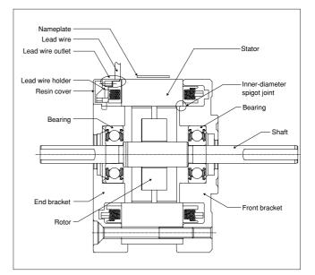
Fig. 3 Motor Structure
